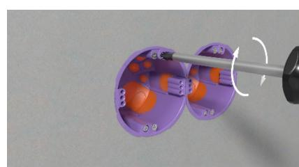
Insert the boxes into the drilled holes and tighten the screws.
