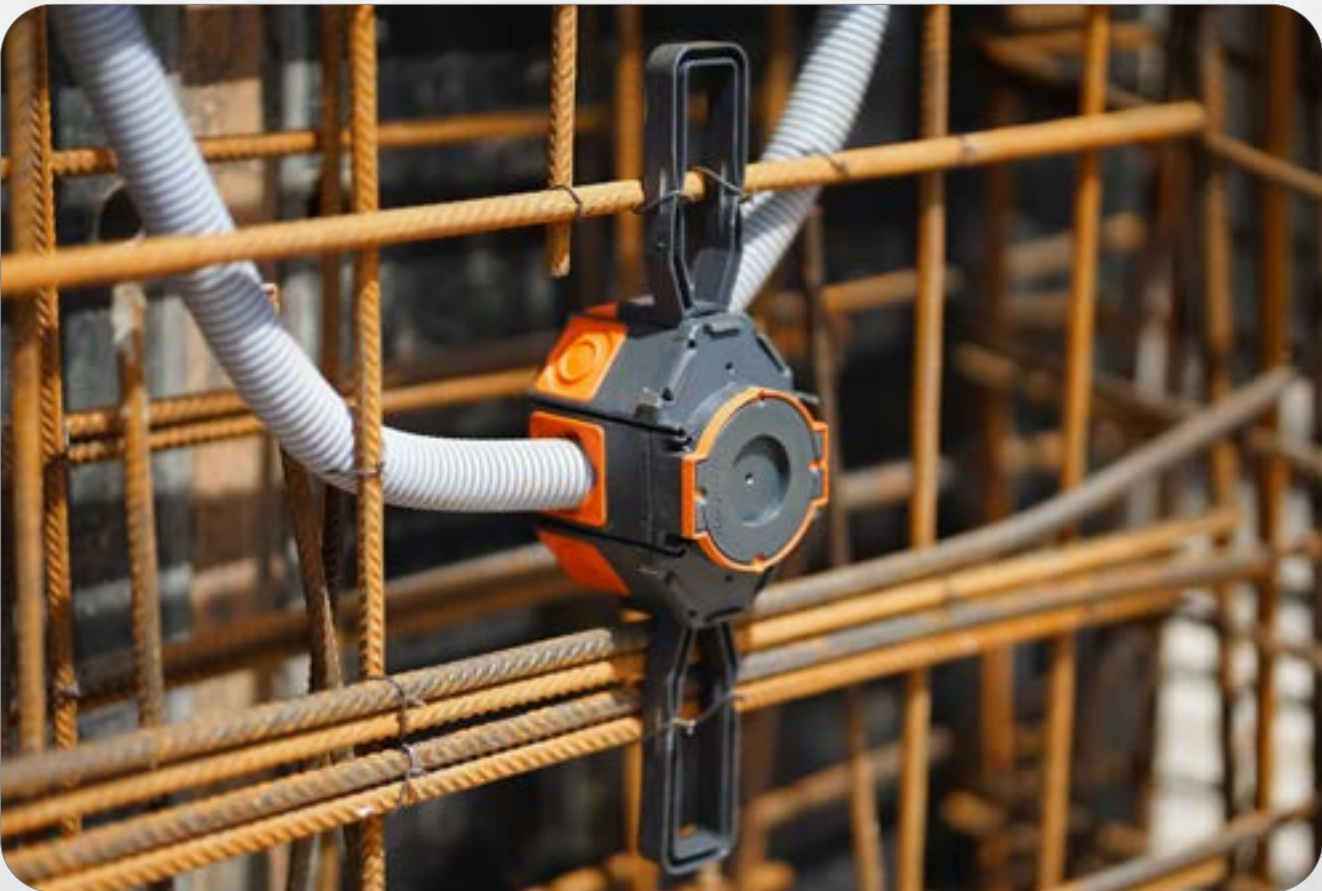
2. Flexible Wings adapt themselves to the respective concrete cover. Concrete covers of 20 – 40 mm or 40 – 60 mm. Concreting can take place after placement of the opposing formwork.
