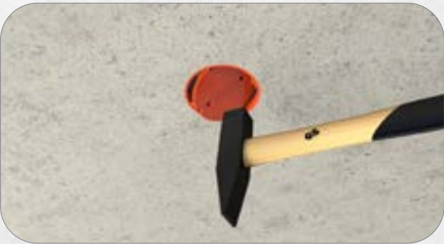
4. Close the box with the cover and concrete the ceiling. Tap in the Front part with a hammer after concreting.
