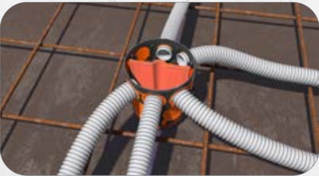
3. Insert cables or (rigid) conduits M40 without tools. Reliable strain relief due to conduit grip. Optional dividing web for two isolated circuits in one box.
