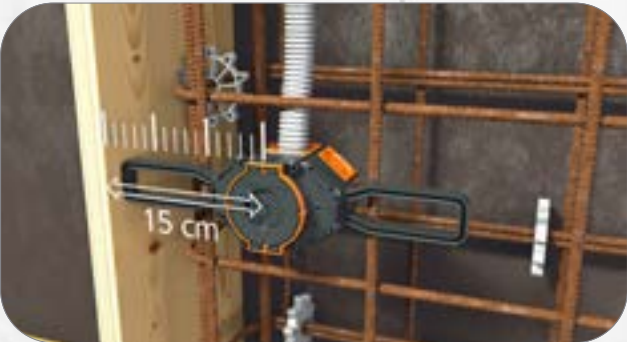
1. Push wings onto the membrane box M1, M2 or M3. Wings set the 15 cm standard distance to door formwork and enable easy mounting. Fasten the wings to the steel reinforcement with wire.
