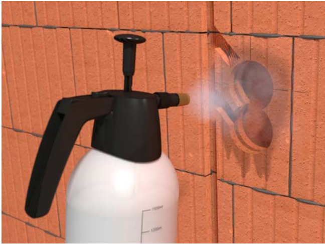
Moisten the hole so that the foam swells better.
