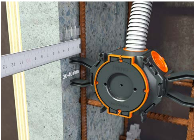
The wings can be pushed on on both sides and are suitable for concrete covers from 20 – 40 mm...
