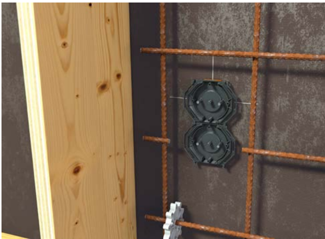
Any number of covers can be connected in-line in a combination spacing of 71 mm.
