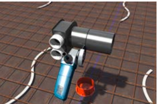
Shorten the nozzle to the desired length.
