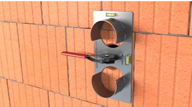
Insert the Drilling template into the existing hole and align it. Clamp with the lever and drill further holes.
