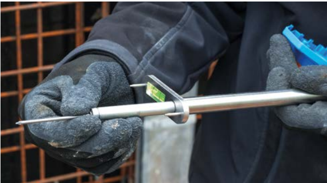
Pick up the nail with the magnet.
