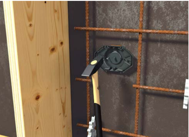
Fasten the cover to the formwork with nails. The integrated nail holder in the cover enables simple installation.
