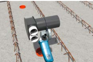
Shorten the nozzle to the desired length and push it into the sleeve.
