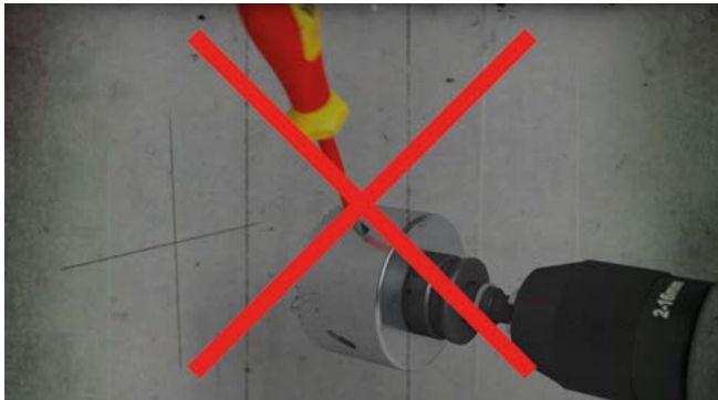
Conventional and time-consuming removal of the core drilling.
