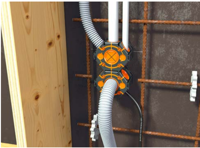
Combination entry of further cables and conduits M15 - M32 without tools. Entry of rigid conduits possible.
